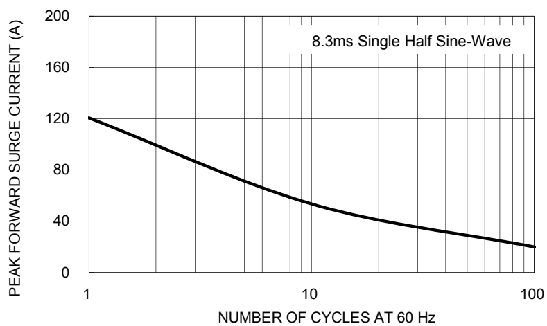
FIG. 3 MAXIMUM NON-REPETITIVE FORWARD SURGE CURRENT
